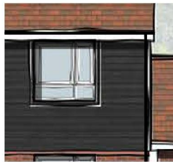
Black Weatherboarding and Metal Frame
